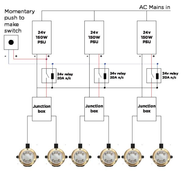
**NOTE:** All relays should be at least 20A contact rated, normally closed type. Pressing switch should disconnect supply to lights.
