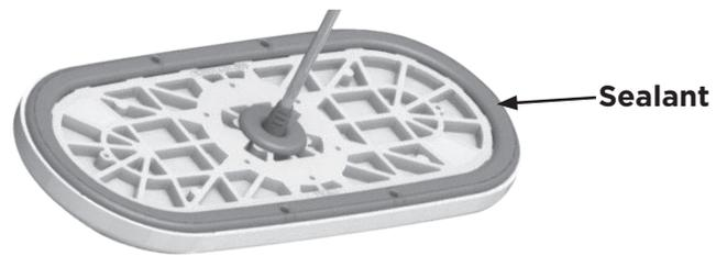
Insert the light on to the hull, feeding the cable through first and seat into place. Press the light hard into the hull and ensure good adhesion.
