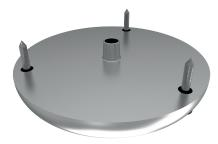
Insert the light on to the hull, feeding the cable through first and seat into place. Press the light hard into the hull and ensure good adhesion. To ensure correct dispersion of light underwater, ensure all Sport Lights are mounted with the correct orientation with text facing upwards. Tip: During/after fitting process, ensure cable is not under any undue stress.
